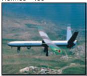
The Hermes 450 is a medium size **UAV** supplying real time intelligence data to ground forces. The UAV (length 6.1 m, wingspan 10.5 m and weight 450 kg), was designed for tactical long endurance
