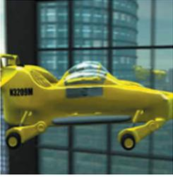
many existing methods. Some of the future prospects include enabling rescue from high-rise buildings and aerial police pursuit of ground targets. The X-Hawk is expected to be able to achieve a maximum speed of 125 mph and fly for up to an hour and a half non-stop.
